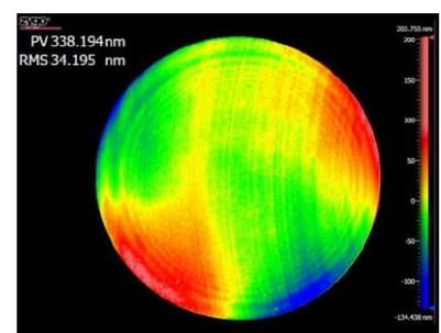
Fig. 3. Interferometer measurement of the telescope, showing a WFE of 34nm RMS.
