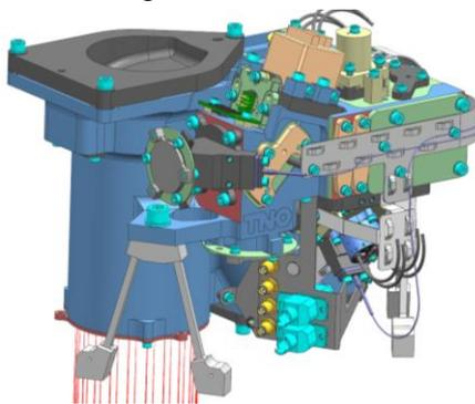
Fig. 1. Overview of the opto-mechanical design of the LEOCAT optical head
