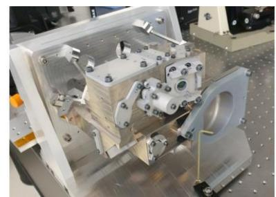
Fig. 2. Photo of the assembly of the LEOCAT optical head
